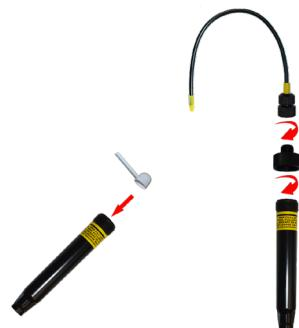
3. Fill powder chamber to max fill line. Then screw on the powder chamber cap and flexible nozzle. **(Keep powder chamber at a 45° angle during filling).**
