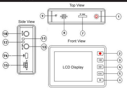
To turn on Mini DVR, ensure the mode switch (standby) is set to position "N", the power button must be then be held for 10 seconds until the blue light illuminates and the screen turns on.
